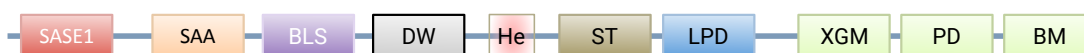
Figure 3.4: Sketch of the beamline layout of the FXE experimental hutch [7]. SASE1: undulator tunnel (see figure 3.3). The components in the FXE experimental hutch are (from left to right): SAA: solid attenuator assembly. BLS: Be lens system. DW: diamond windows as separation between the accelerator vacuum and the experimental area in air or helium atmosphere. He: helium section to sample stage. ST: sample stage. LPD: large pixel detector with beam path in air. XGM: prototype gas monitor detector with beam path in Xe atmosphere. PD: stage with calibrated photo diodes from PTB [11]. BM: room temperature radiometer from AIST as primary standard [8–10].
