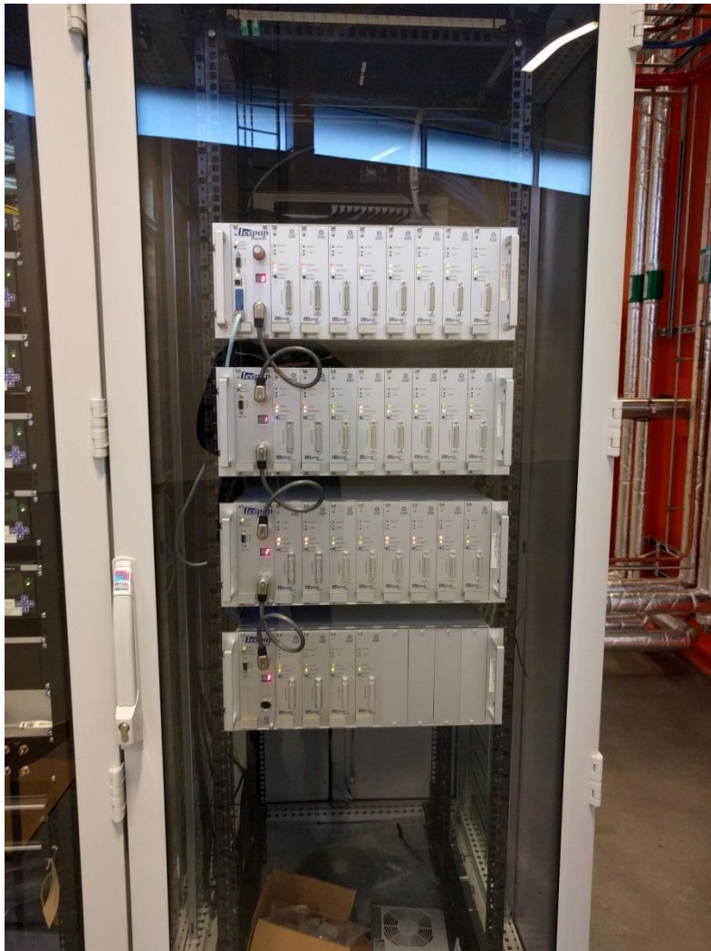
Figure 4: Icepap module in a 19-inch module frame
